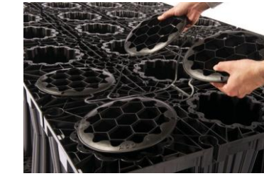
Recycled polypropylene top covers are added to the top layer of the system to ensure consistent vertical support for the cover fill material.
